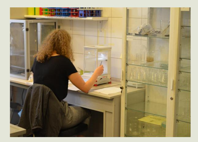
Laboratory of soils, rocks and sediments micromorphology (here are made thin microscopic slides of soil (also rocks) hardened with resin, ground to transparency, allowing its micromorphology to be examined
